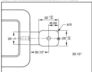
Note: When the core pin is not shutting off on the inner core wall, the distance from the edge of the insert should be 29.00 for the slide carrier to shut off against the core insert.
