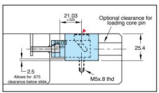
Note: 21.03 dimension must be maintained to avoid improper spring pre-load or damage to internal components.
